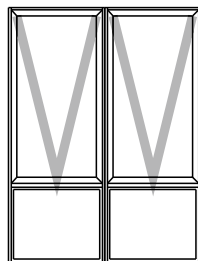
Double awning over double fixed light
